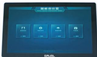
GFC-2782LC: 桌面式有线触摸屏(15.6寸)
